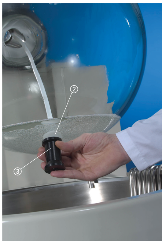
Fig. 4.17: Positioning the tip of the hose with the magnet
