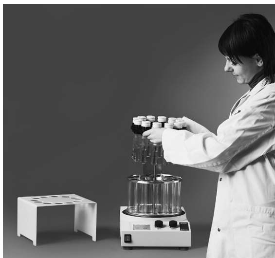
Fig. 4.13: Simultaneous sample transfer using the transfer plate
