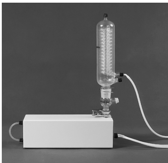
Fig. 4.20: Cooled receiver with type S condenser
