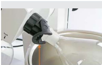
EASY CLIP open, flask unclamped
