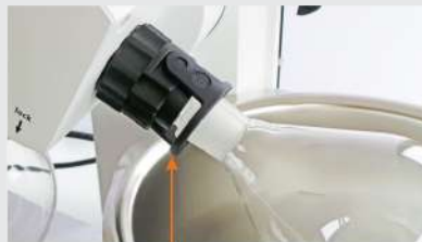
EASY CLIP closed, flask clamped
