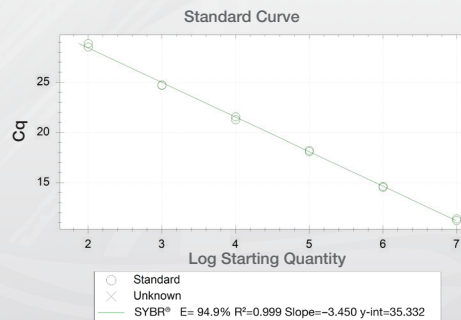
Figure 3: A standard curve can be generated with a serial dilution of template DNA. An inverse correlation exists between the log of the quantity of DNA (x-axis) and the C q value (y-axis). PCR efficiency can be calculated from the slope of the standard curve and utilized for calculating relative quantity (Pfaffl Method).
