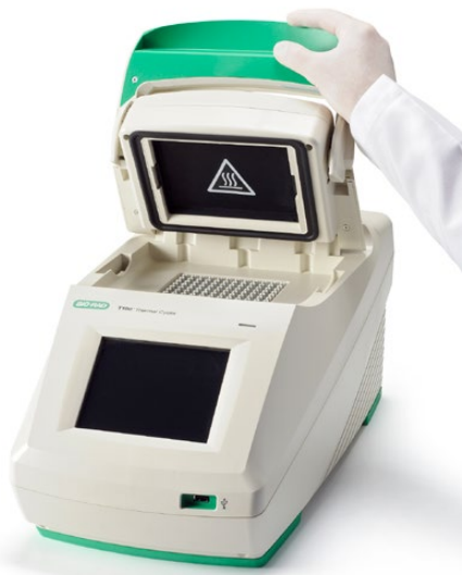
Fig. 3. Lift the lid handle up to open the lid.
